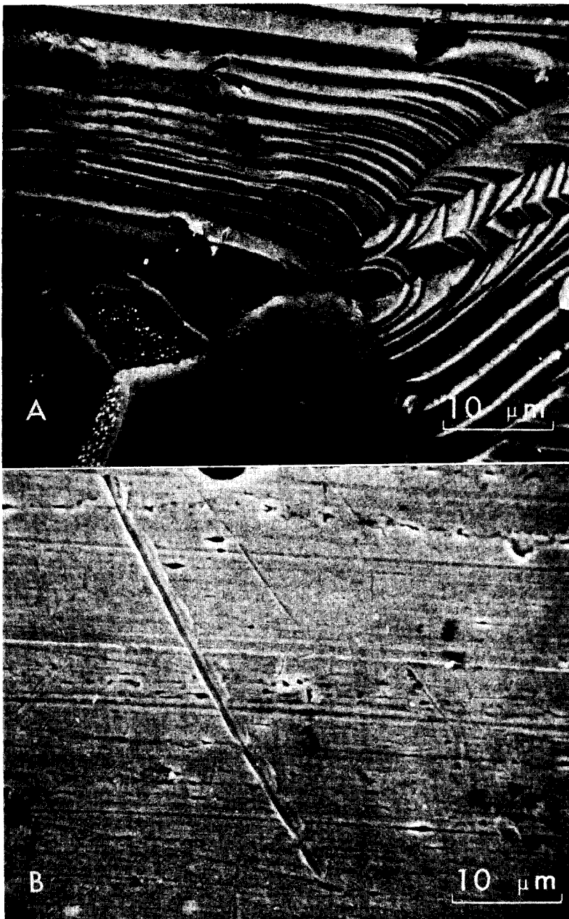
FIG. 1. Surface topography of (A) thermally etched silver and (B) polycrystalline silver.
